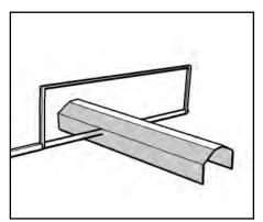
The gutters have to be cut in the correct length. PVC gutters can be cut easily with a small saw. Make sure the cut is straigth and clean. If necessary, you can clean the cut with a knife or a piece of sandpaper. Also wipe off remaining sawdust from the gutter.
