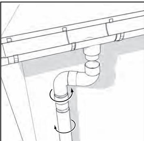
With elbows you can guide the downpipe from the gutter outlet to the wall. Connect the downpipe and elbow by using glue.
